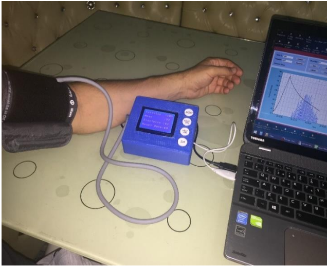
Fig. 7. The developed prototype for blood pressure and heart rate measurement
