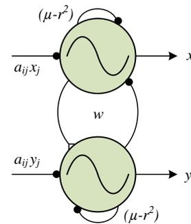
Fig. 2. Hopf oscillator structure
