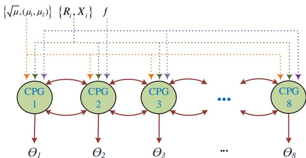
Fig. 5. CPG network structure with bidirectional coupled scheme
