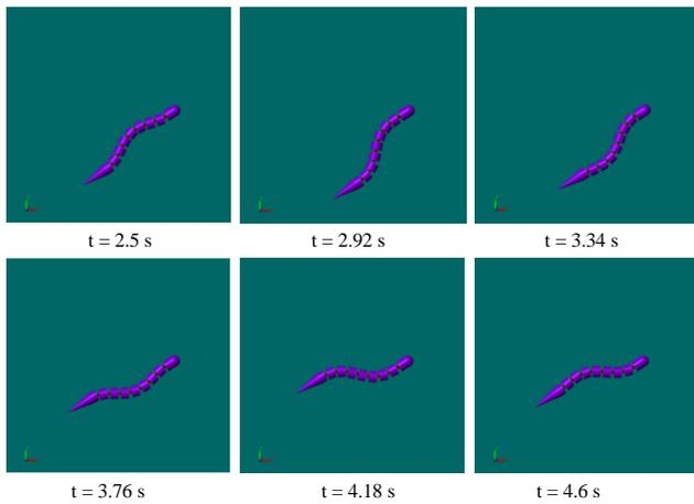
**Fig. 7.** Snapshots of SimMechanics analysis for forward motion of the snake robot
