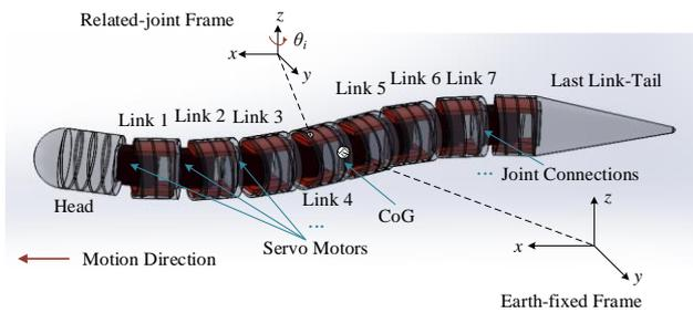
Fig. 3. The designed snake robot model
