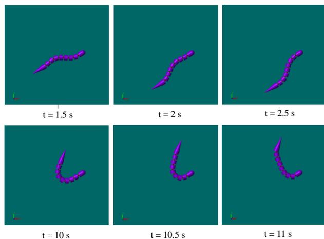
**Fig. 10.** Snapshots of SimMechanics for forward and turning motions of the snake robot. It is noticed that After 10 s, bias is set to 1.25
