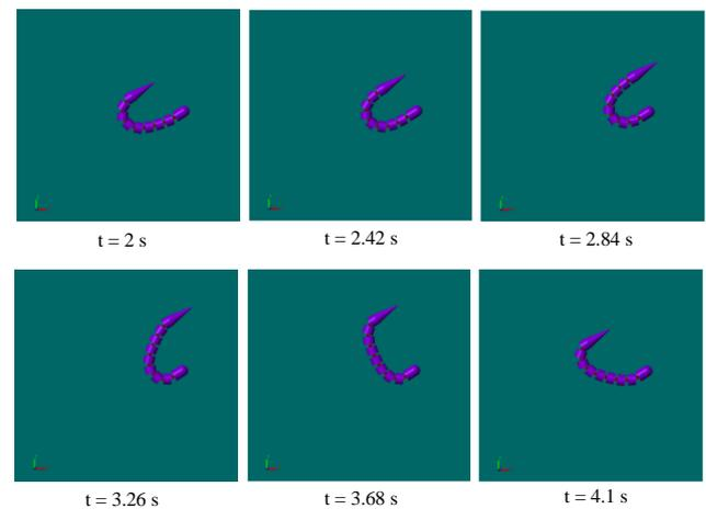
**Fig. 9.** Snapshots of SimMechanics analysis for turning motion of the snake robot
