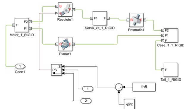
Fig. 4. MATLAB/SimMechanics model of a link of the snake robot
