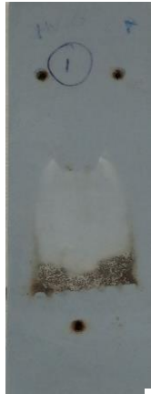
Fig. 12. Test Sample-A after the IPTE test
