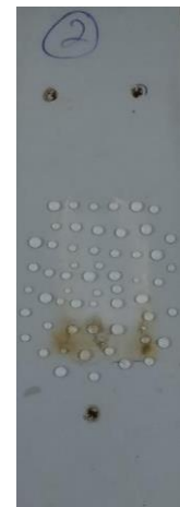
Fig. 17. Water droplets on Sample-B, 48 hours after the IPTE test
