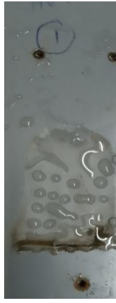
Fig. 13. Water droplets on Sample-A immediately after the IPTE test
