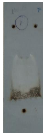
Fig. 15. Test Sample-B after the IPTE test
