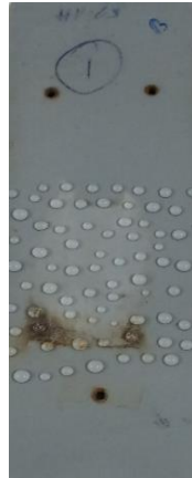
Fig. 14. Water droplets on Sample-A, 48 hours after the IPTE test
