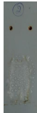
Fig. 16. Water droplets on Sample-B immediately after the IPTE test
