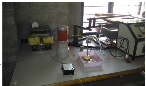
Fig. 3. Experimental test set-up for inclined plane test.
