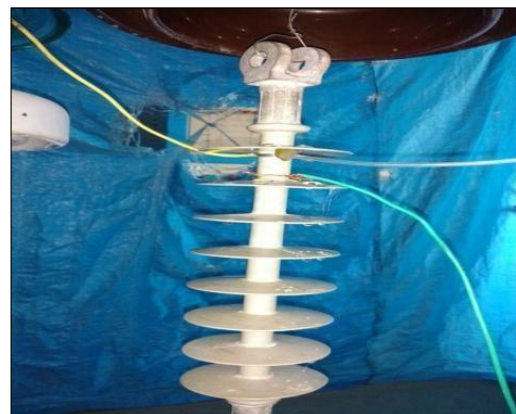
Fig. 10. Experimental set up on a section of 66kV polymeric insulator
