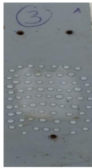
Fig. 20. Water droplets on Sample-C, 48 hours after the IPTE test
