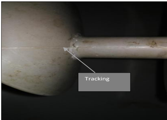
Fig. 11. Tracking on a section of 66kV polymeric insulator after Inclined Plane Test.
