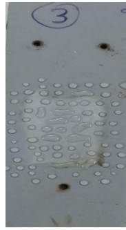
Fig. 19. Water droplets on Sample-C immediately after the IPTE test
