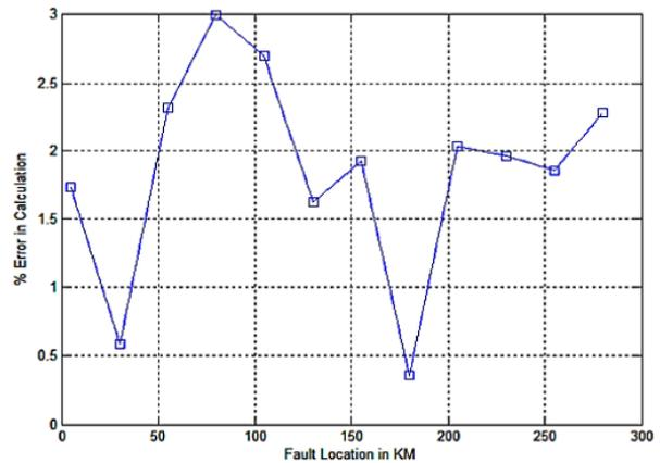
**Fig. 8.** (6-21-1) Configuration ANN Test Phase Performance
