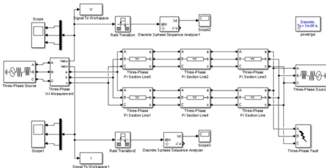
**Fig.2.** EHV transmission line simulation model
