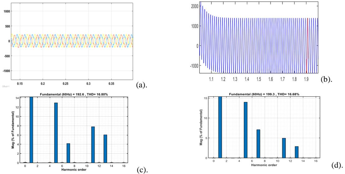
**Fig 10.** (a) Load current ( $I_L$ ), (b) Load voltage ( $V_L$ ), (c) THD analysis using FFT window of load current ( $I_L$ ), and (d) THD analysis using FFT window of load voltage ( $V_L$ )
