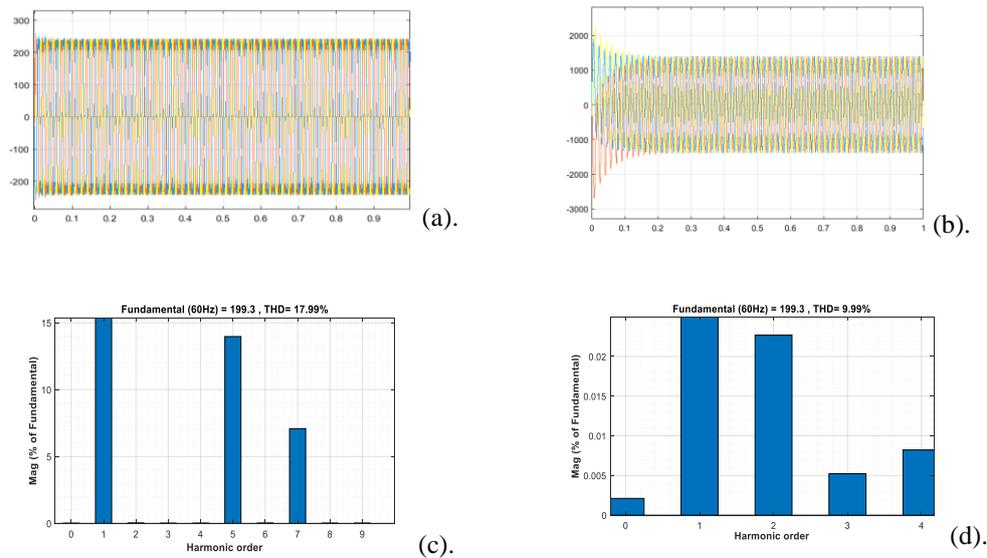
**Figure 11.** (a) Load current ( $I_L$ ), (b) Load voltage ( $V_L$ ), (c) THD analysis using FFT window of load current ( $I_L$ ), and (d) THD analysis using FFT window of load voltage ( $V_L$ )
