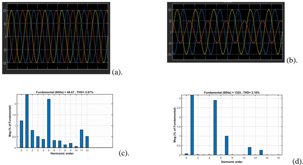
**Fig 13.** (a) Load current ( $I_L$ ), (b) Load voltage ( $V_L$ ), (c) THD analysis using FFT window of load current ( $I_L$ ), and (d) THD analysis using FFT window of load voltage ( $V_L$ ).
