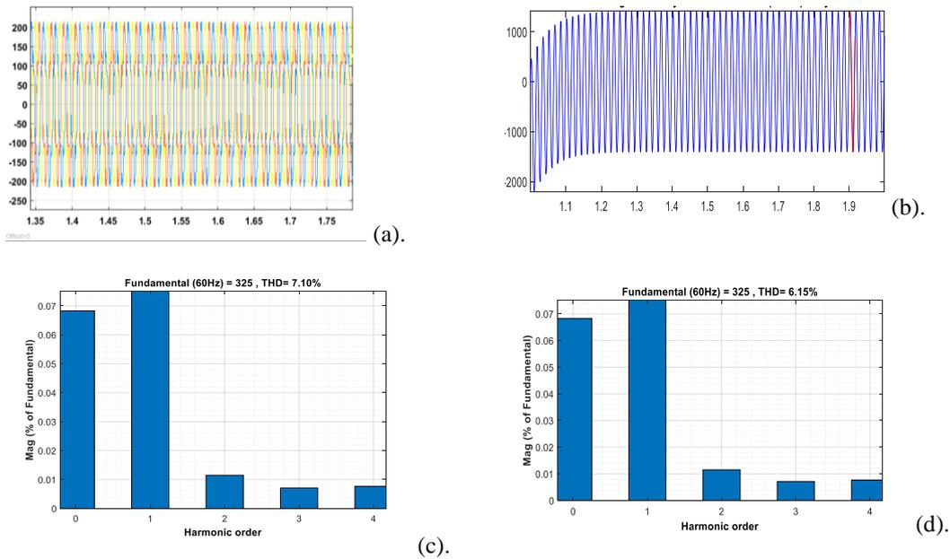
**Fig 12.** Load current ( $I_L$ ), (b) Load voltage ( $V_L$ ), (c) THD analysis using FFT window of load current ( $I_L$ ), and (d) THD analysis using FFT window of load voltage ( $V_L$ )
