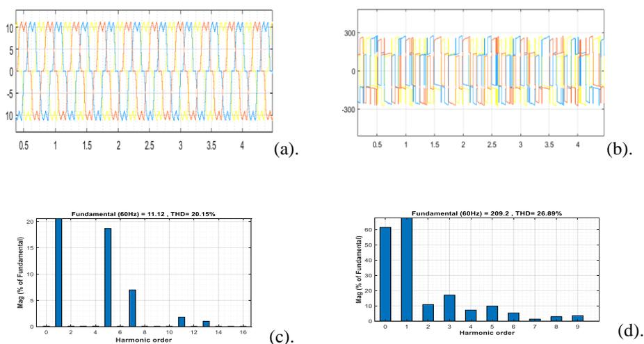
**Fig 8.** (a) Load current ( $I_L$ ), (b) Load voltage ( $V_L$ ), (c) THD analysis using FFT window of load current( $I_L$ ), (d) THD analysis using FFT window of load voltage ( $V_L$ )
