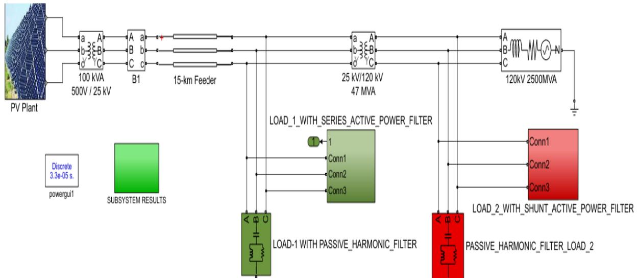
Fig 4. Simulation Setup of the proposed model in MATLAB toolbox
