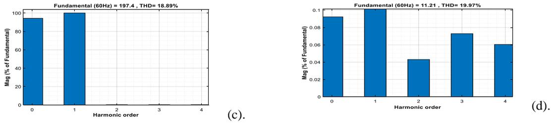
**Fig 9.** (a) Load current ( $I_L$ ), (b) Load voltage ( $V_L$ ), (c) THD analysis using FFT window of load current ( $I_L$ ), (d) THD analysis using FFT window of load voltage ( $V_L$ )
