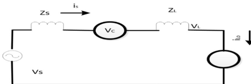
Fig 3. Series APF with harmonic voltage load
