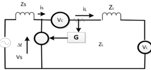
Fig 5. Shunt APF for the harmonic voltage load
