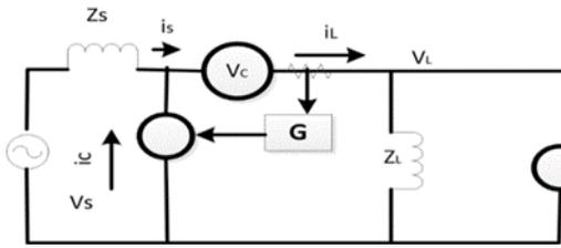
Fig 4. Shunt APF for harmonic current load
