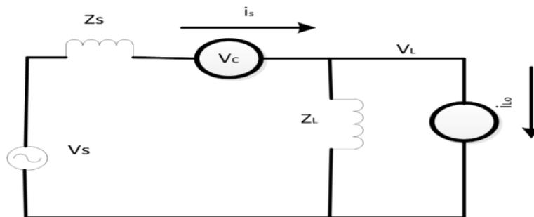
Fig 2. Series APF for the harmonic current load
