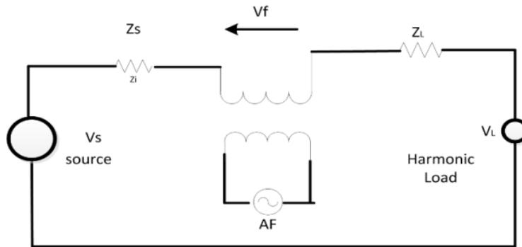
Fig 1. A Series Active Power Filter
