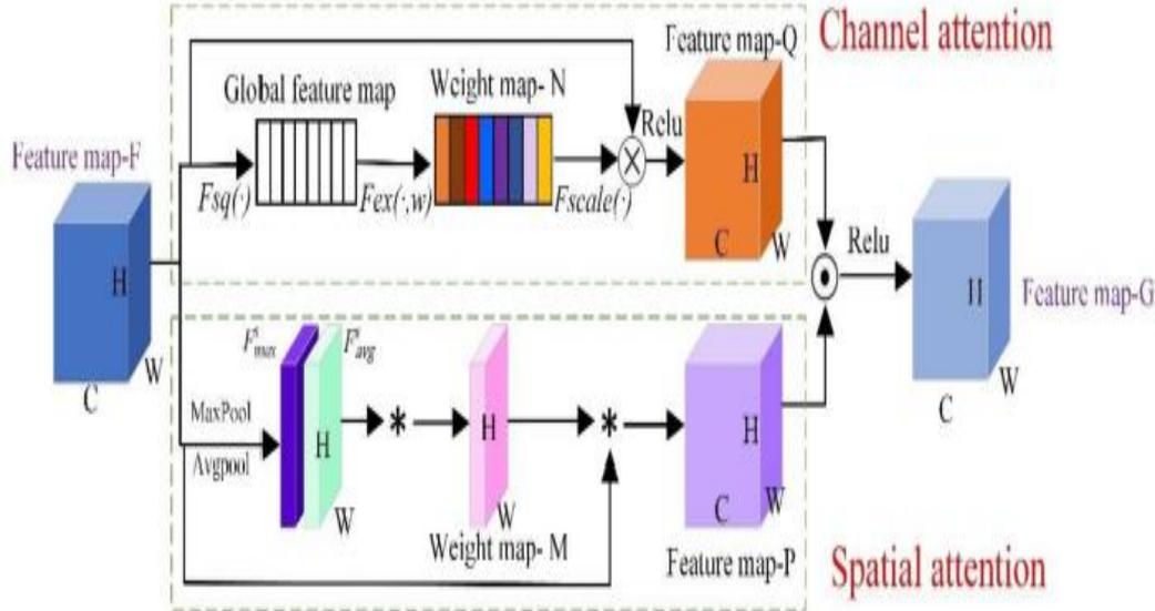
Fig. 4. Improved CNN structure of the parallel attention mechanism
