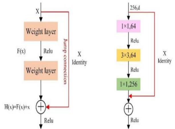
Fig. 5. The residual block (left) and the bottleneck structure (right)
