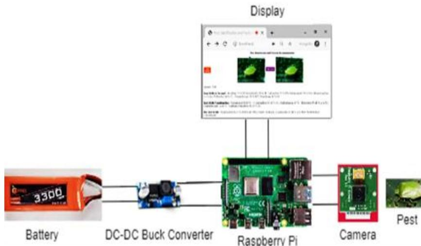
**Fig. 11.** Experimental Setup of Pest Identification
