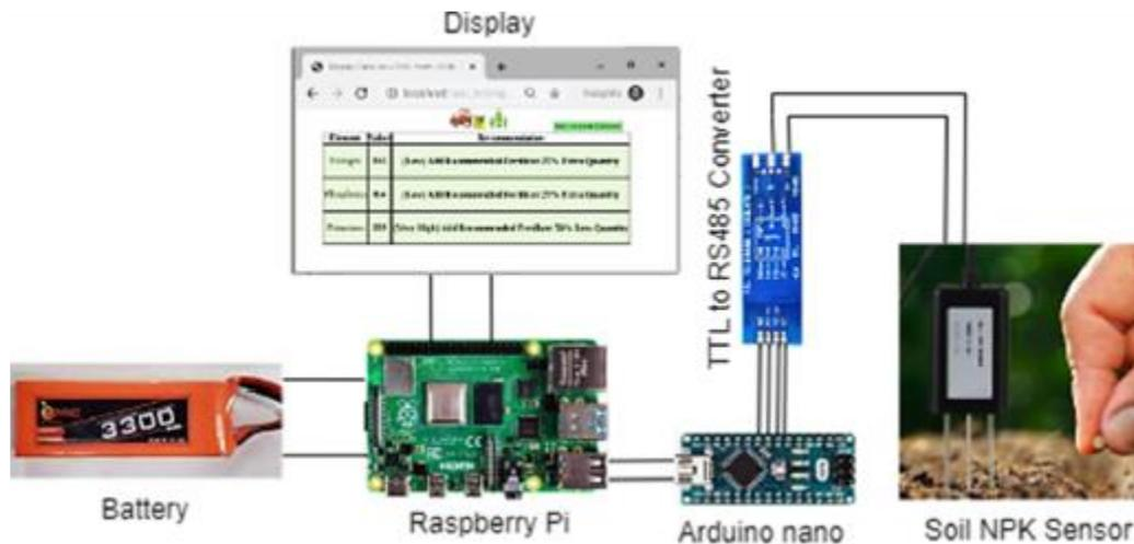
**Fig. 14.** Experimental Setup of Soil NPK Value Data Collection
