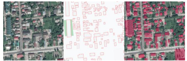
Fig 14: Google Maps Satellite view, Google Maps' view, Extracted Building Masks from google maps (left to right)
