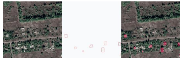
Fig 16: From left to right, the text describes Google Maps Satellite view, Google Maps view, and Extracted Building Masks from Google Maps
