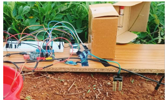
Fig 7. Device used to connect IoT sensor with Arduino.
