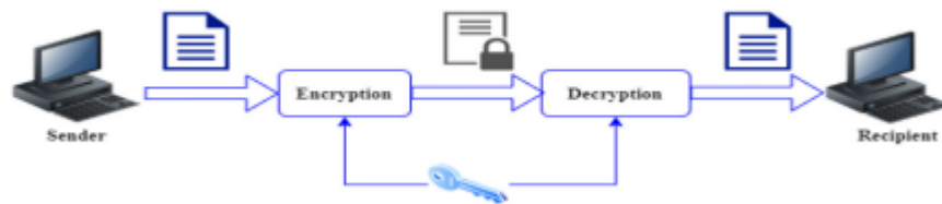
Fig 2. Symmetric key encryption
