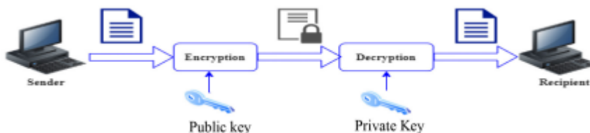
Fig 3. Asymmetric key encryption [22]
