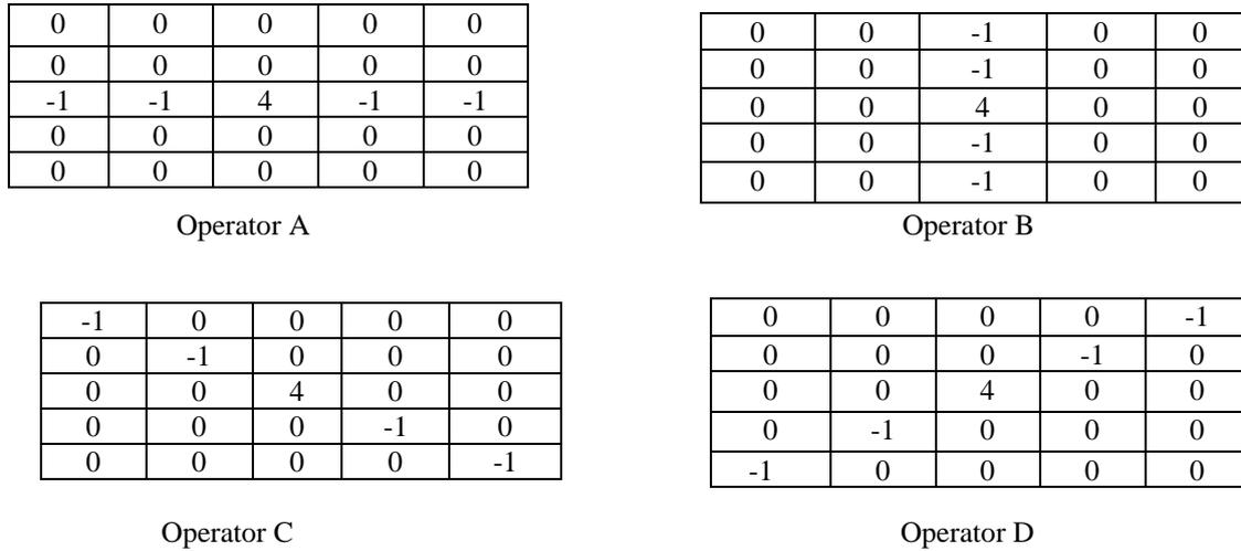
Fig. 2 Four Laplacian operators
