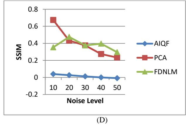
**Fig. 6** Demonstrate performance of image denoising techniques in Terms of SSIM for the datasets (A) Lena, (B) Mandrill (C) Women (D) Camera man
