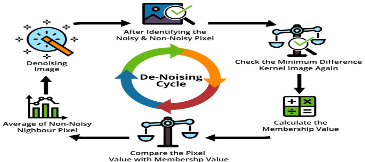
Fig. 3 Procedure of the hybrid AIQF model using fuzzy membership
