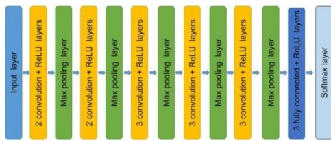
Fig 5.2: The architecture of VGG16 [1]
