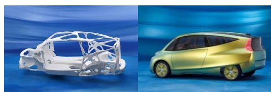
Fig 1. DaimlerChrysler's electric car is inspired by the growth patterns of trees and box fish [6]
