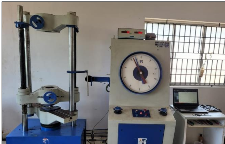
Fig. 4. Experimental setup of Compression Testing Machine
