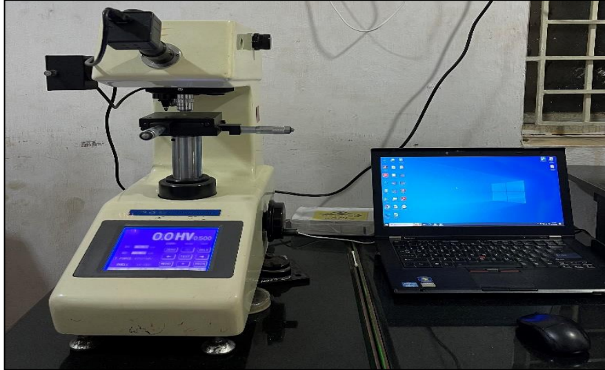
Fig. 3 Experimental setup of Vickers hardness testing machine
