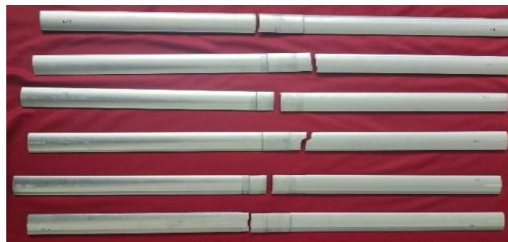
Fig. 11. MPW Specimen after Tensile Fracture
