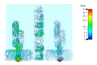
Fig.12.(c) surface current at 4.5 GHz.
