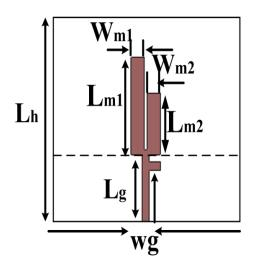
Fig.1 Antenna frond Design
