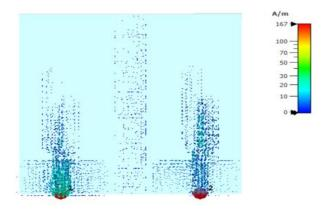
Fig.12(b). Surface current at 2.4 GHz
