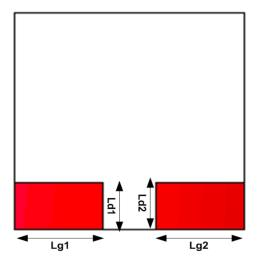
Fig.2(a) Back side of the mimo antenna
