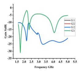
Fig.7. Unit cell s- parameter simulattion Result
