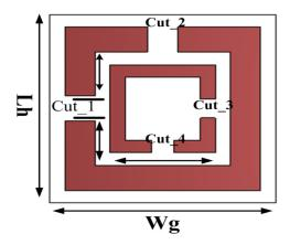
Fig.6. Metamerial unit cell.
