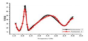
Fig.4. VSWR Results in proposed antenna
