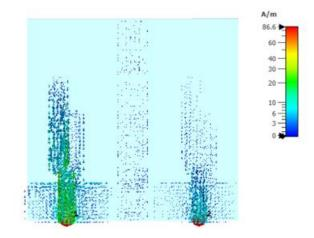
Fig .12(a). surface current at 1.8 GHz
