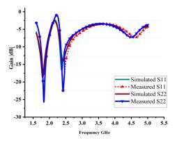
Fig.3 S-parameter simulation and Measured Result
