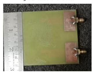
Fig.10 fabricated antenna back side
