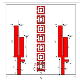
Fig.2.MIMO antenna Design
