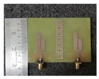
Fig.9. fabricated antenna front side
