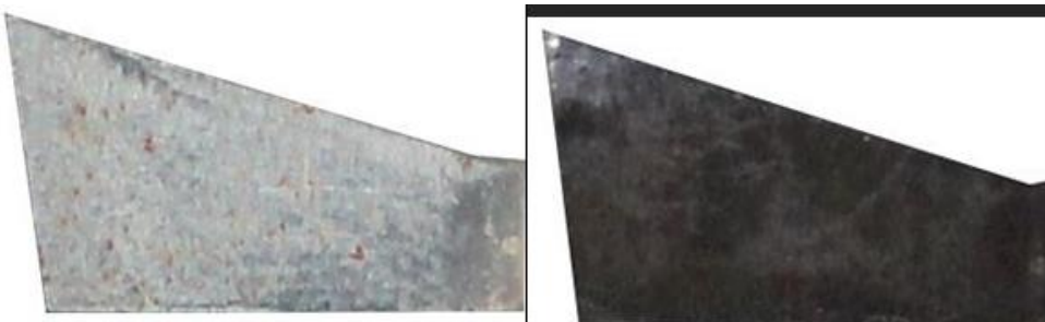
Figure 9. Tool-8 geometry before and after experiment
