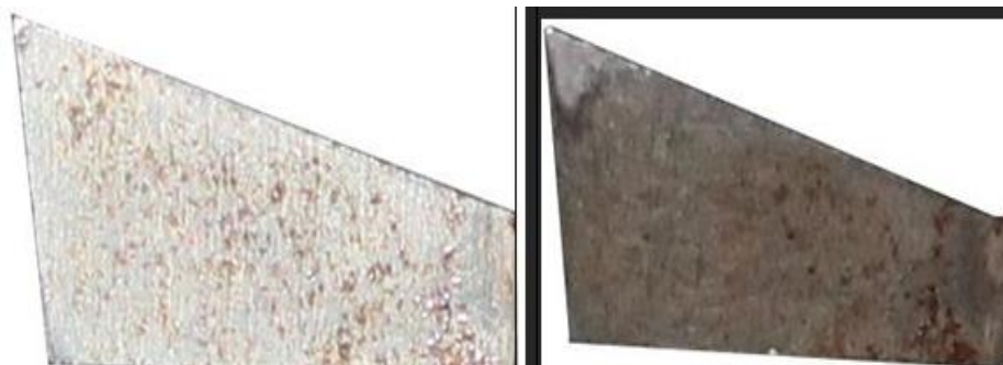
Figure 5. Tool-4 geometry before and after experiment
