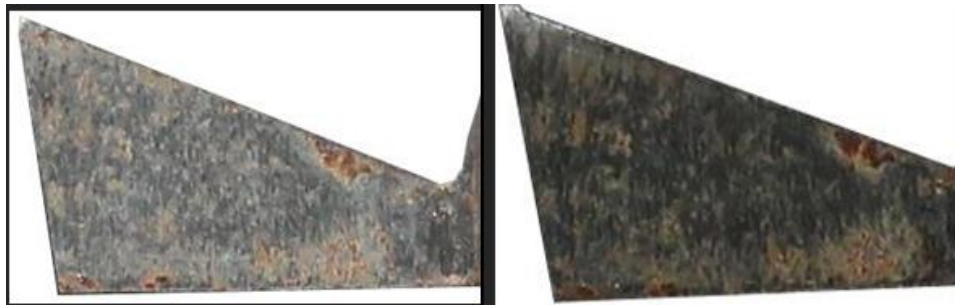
Figure 12. Tool-11 geometry before and after experiment
