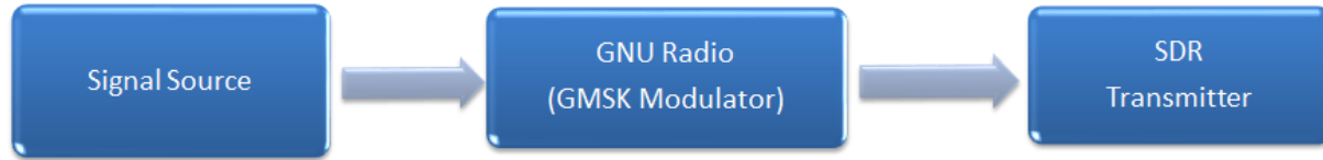
Figure 3a: block diagram transmitter for energy based spectrum sensing
