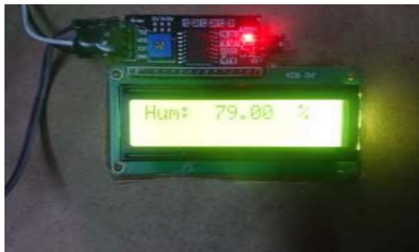
Figure 6: LCD Showing the Humidity value
