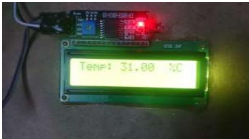
Figure 5: LCD Showing the Temperature value
