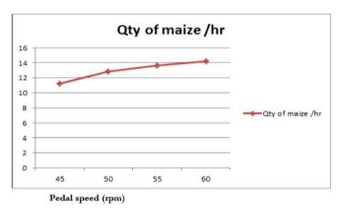
The quantity of maize threshed by the thresher increases with the increase in pedal speed as the blade speed increases. Result for motor operated Mechanism
