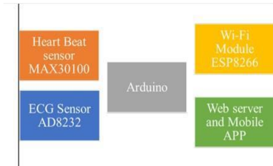
Fig. 2 shows the design of the IoT device-based ECG system[1]
