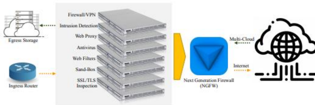
Fig. 2. An architecture for the future generation of firewalls that is data-driven for SD-WANs.
