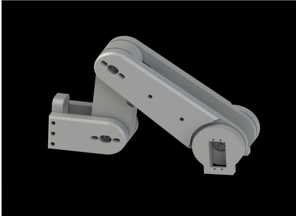
Figure 2. CAD render of the open-source-derived articulated arm used for the prototype.
